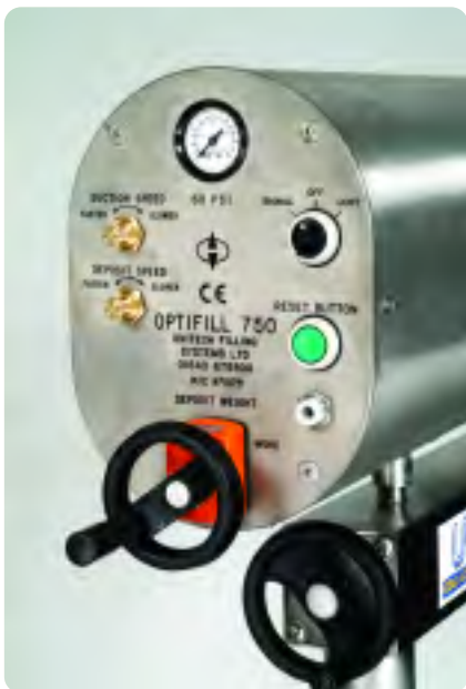
■ Left: The operating panel is easily accessible at the rear of the depositor. Deposit weight, deposit speed and suction speed are readily adjustable. The depositor can be operated either in continuous mode (mainly for priming) or in signal mode, using a footswitch or a signal from a conveyor.
