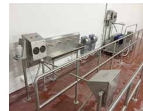
Typical Hygiene Entrance Arrangement
