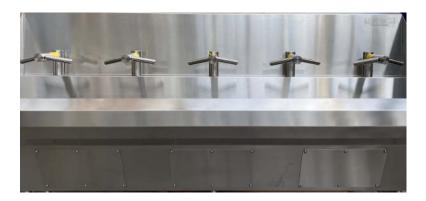
Our client, one of the UK's largest seafood processors, asked us to design a sink incorporating Dyson Airblade wash and dry tap assemblies into our stainless steel hygiene sinks.
