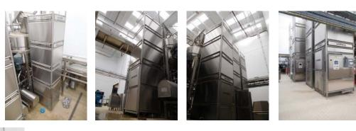
Unitech Engineering have completed a bespoke project to design, manufacture and install 6 of their tallest lifting and tipping machines yet. The client, Briggs of Burton, a specialist process engineering company, appointed Unitech Engineering to provide a simple solution for lifting and tipping 350kg euro bins containing a variety of products.
