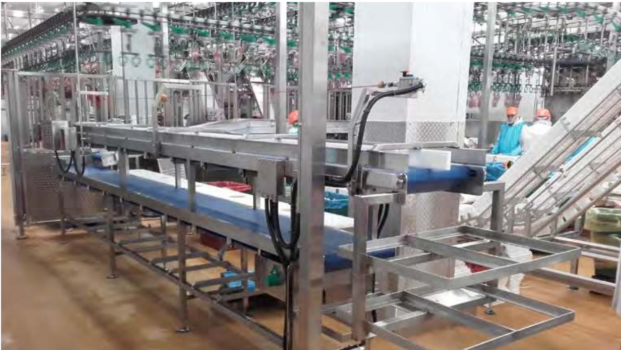
Typical twin tier chicken wing trimming stations, designed around the customer's specific requirements for their labour and product specification.
