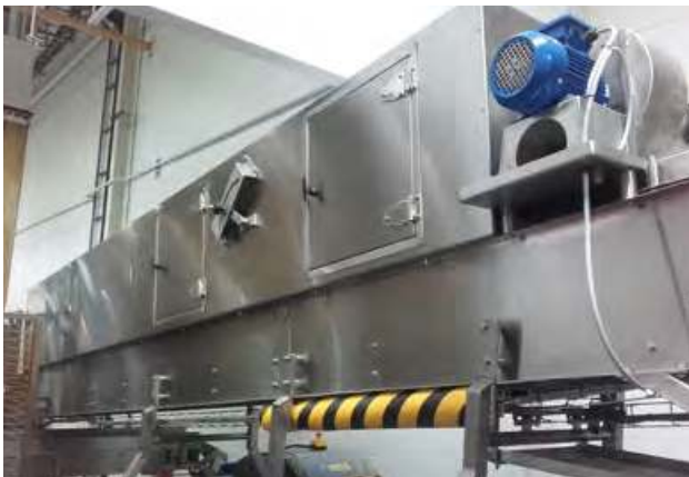
Rice cake cooling complete with laning and separation of the rice cakes. The cooling conveyor reduces the temperature of the cakes from 120°C down to 20°C allowing faster packaging of the product. Rice cakes are very delicate in nature and require smooth handling, all being achieved to the customer's satisfaction.
