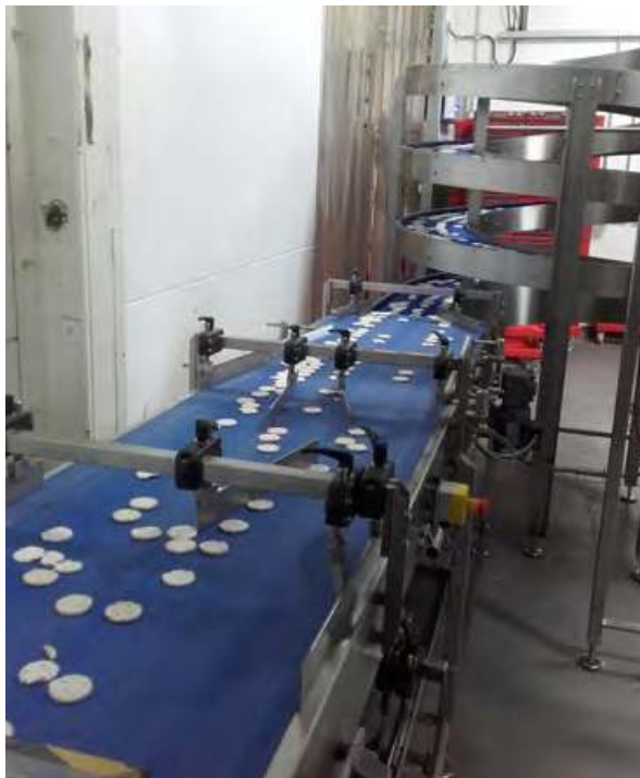
Rice cake cooling complete with laning and separation of the rice cakes. The cooling conveyor reduces the temperature of the cakes from 120°C down to 20°C allowing faster packaging of the product. Rice cakes are very delicate in nature and require smooth handling, all being achieved to the customer's satisfaction.
