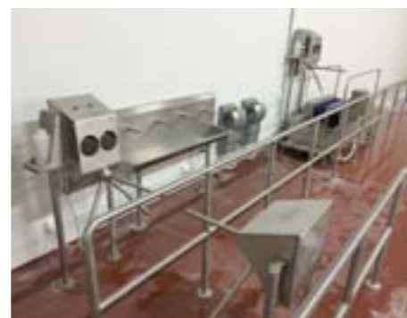
Typical Hygiene Entrance Arrangement
